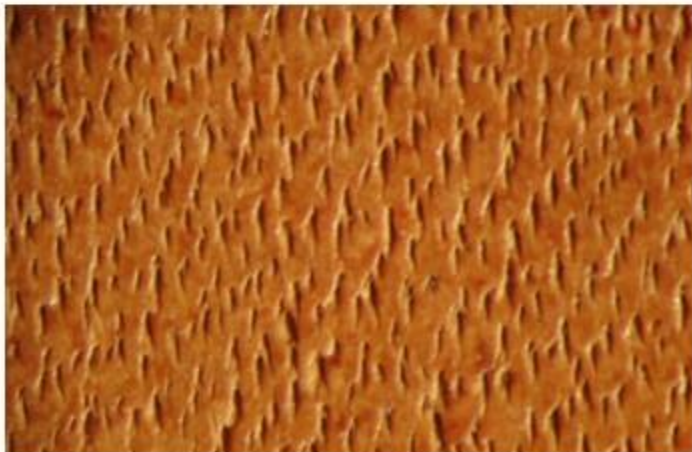
Grain surface of bovine leather (x20 mag).
